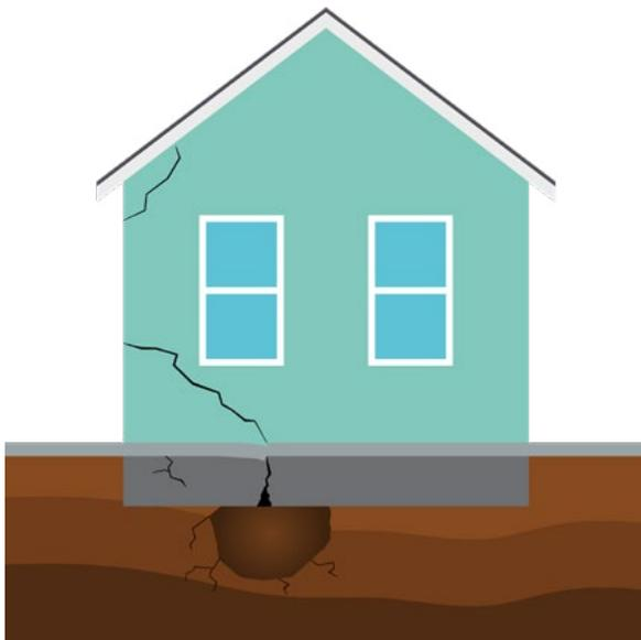
To adequately analyze the building's instability, it is necessary to have regular and constant measures over time. Moreover, sometimes, it is not sufficient the structural control but it is also necessary to monitor the **environmental conditions** and the **surrounding land**.
